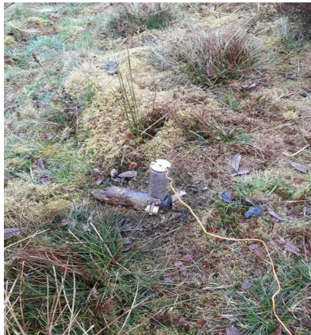
Burning out explosive from a WW2 shell. The burner is fired from a safe distance by the electric initiator.
